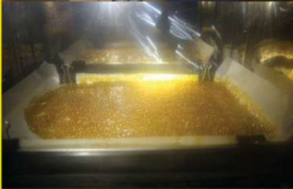
(Above and left) TC Labs uses laboratory vacuum ovens for the next step in the process. The oven introduces heat and pressure to remove the solvent left in the solution. The butane and hash solution will "boil" as the remaining solvent continues to release its bonds.
